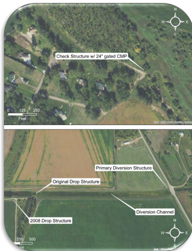
Figure 2: Burnt Creek Flood Control Project Features
