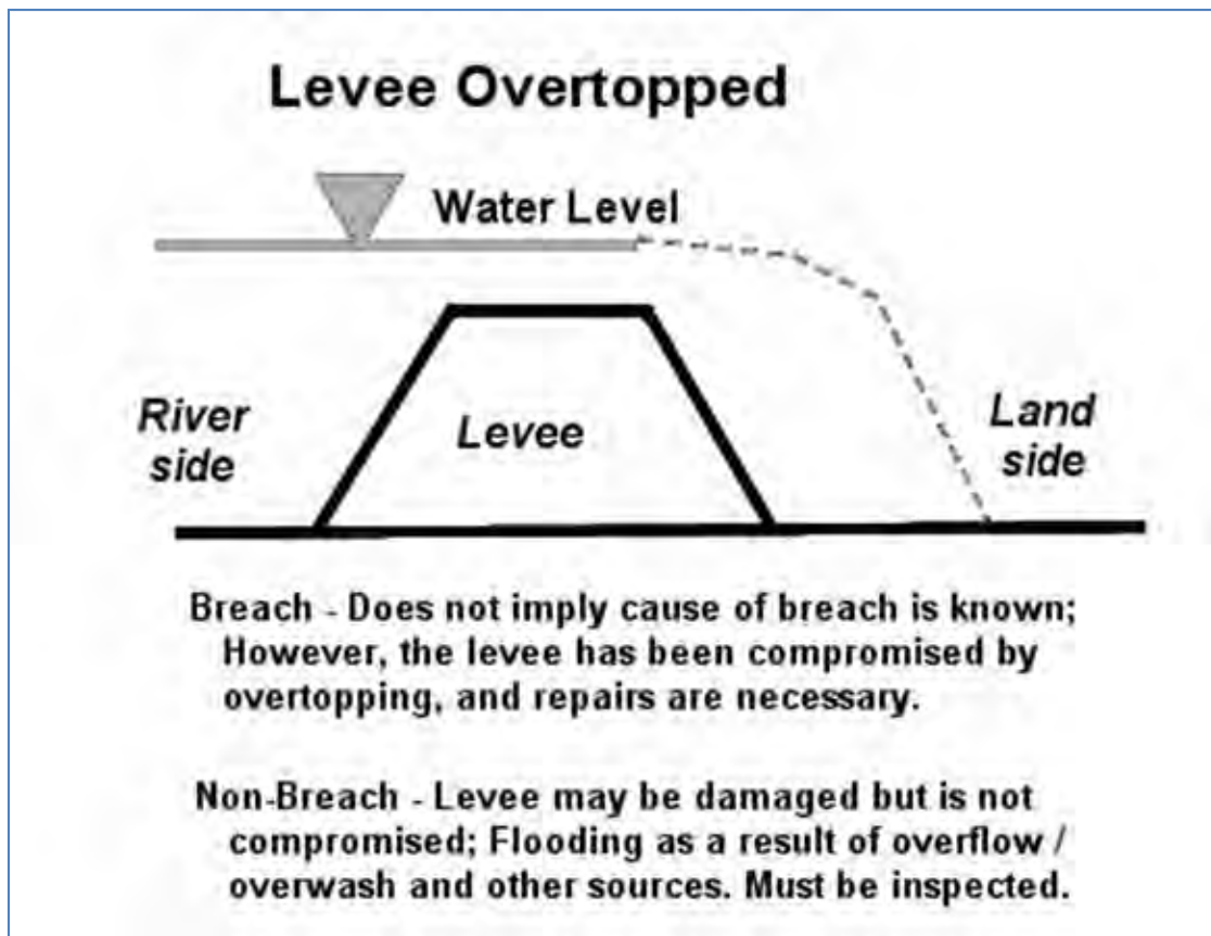
Figure 9 – Possible results when levee is overtopped.
